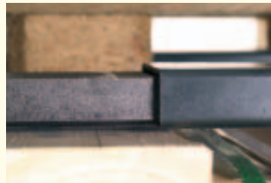
◀ Special design of outerforks prevents damage when forks are being retracted.
